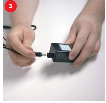
3 TRANSFORMER SHOULD ALREADY BE ATTACHED, IF NOT SIMPLY PLUG CORD INTO TRANSFORMER (MAKE SURE TRANSFORMER IS NOT PLUGGED IN).
